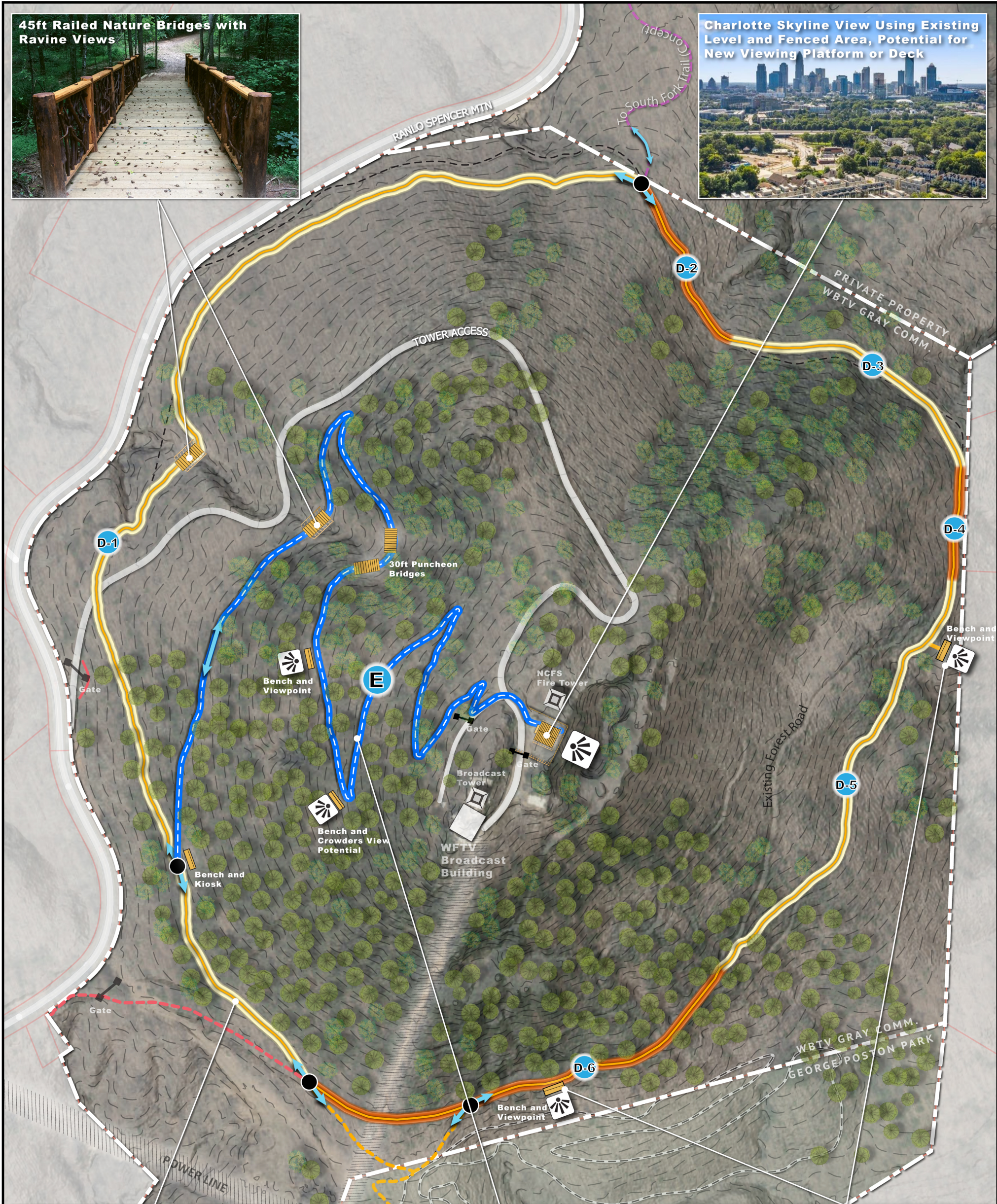
Existing Forestry Road Converted to Contouring Multiuse Trail with Improved Drainage, Realignments, and Gravel Surfacing
