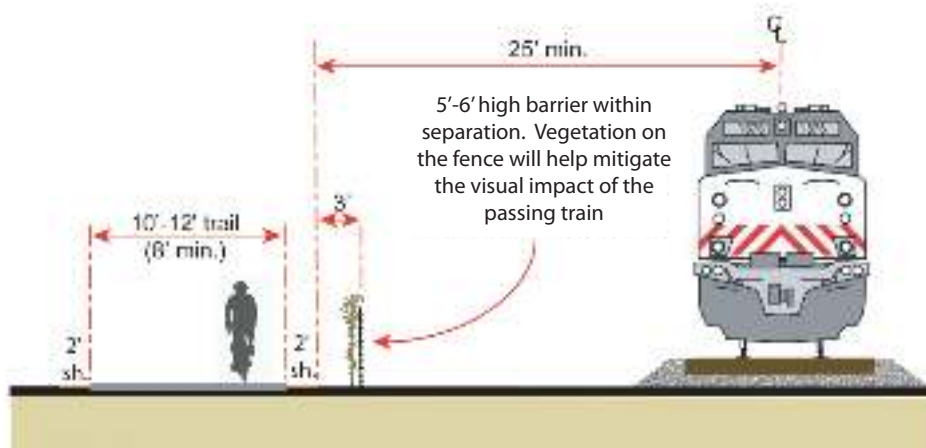
Typical rail with trail section
